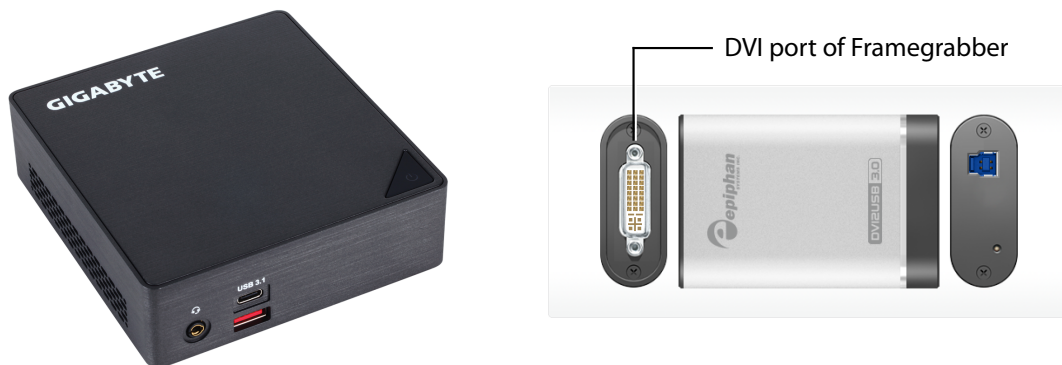
Display Capture Unit: Brix and Framegrabber
