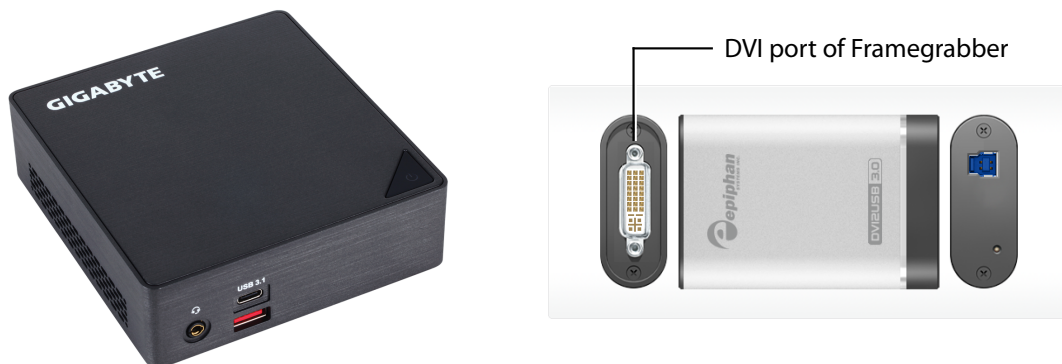
Display Capture Unit: Brix and Framegrabber
